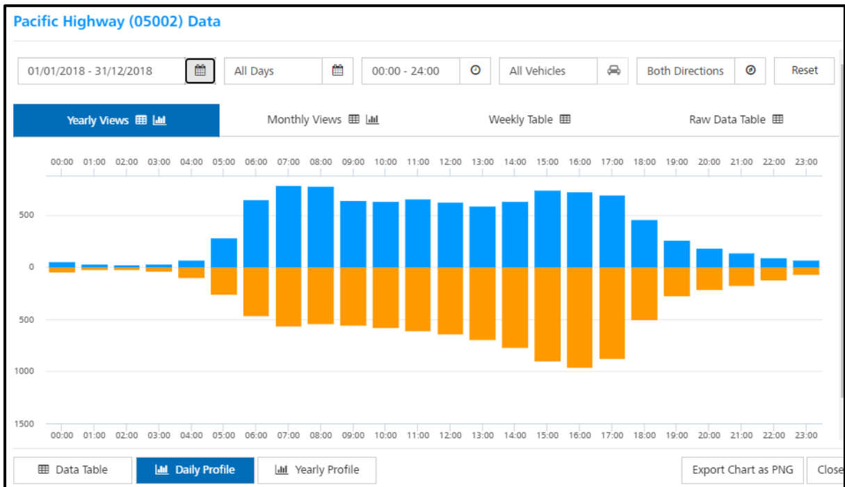
Figure 3-6 Distribution of daily flows on the Pacific Highway (Source: TfNSW Count station 05002)
