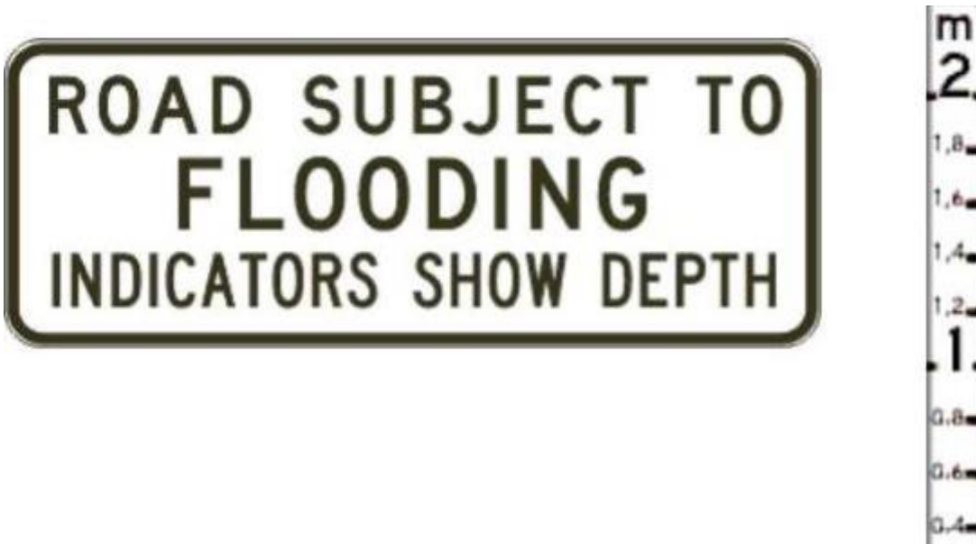
Figure 13 Example Flood Depth Indicator
