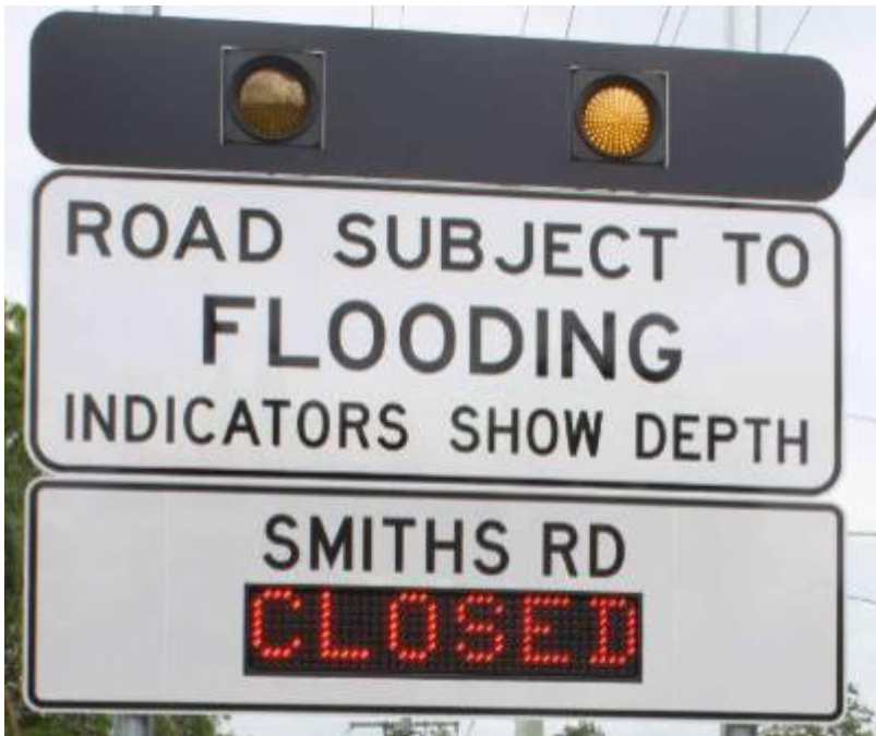
Figure 12 Example Flood Warning Sign
