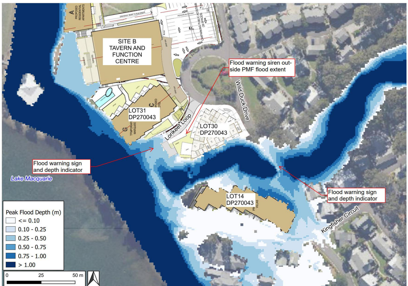
Figure 11 Proposed Flood Warning System
