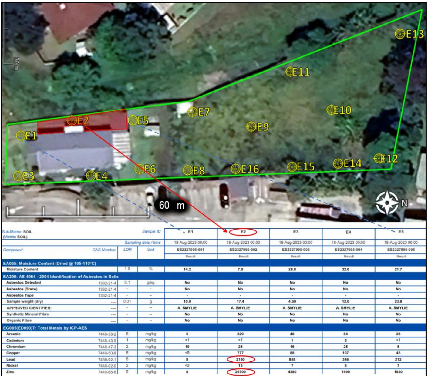
Figure 1. Top image shows sampling areas indicated by yellow alphanumeric labels and targets. The red section highlights an approximation of the remediation area. The red arrow leads to an excerpt of the laboratory certificate of analysis that shows sample E2 yielded levels of lead and zinc that exceed HILs A, and lead that exceeds HILs D (compare with Figure 2). Blue dashed lines indicate samples (E1 and E5) that were used to delineate the expected extent of the remediation area, as they returned contamination levels below ASC NEMP thresholds.
