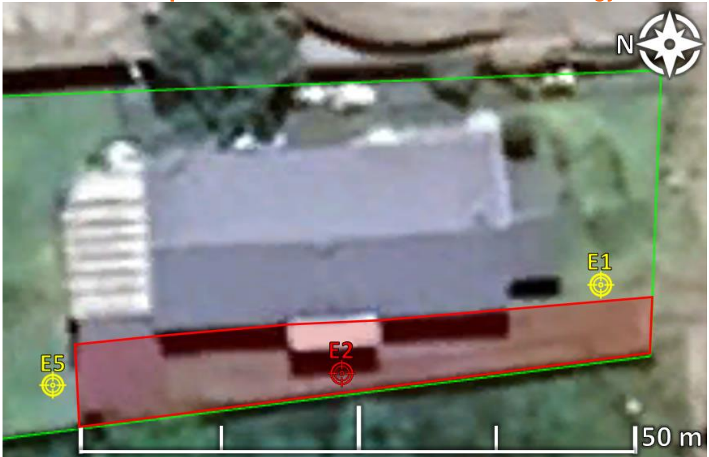
Figure 4. Satellite imagery of the Site with the remediation area in red. The red target and red label E2 indicate where the contaminated sample was obtained. The red boxed area indicates where excavation work is recommended to occur. The yellow targets and alphanumeric labels (E1 and E5) are areas where sampling did not find contamination to exceed HIL thresholds. Sample depths for E1, E2, and E3 were taken at 2 m, 30 mm, and 150 mm, respectively. Green outline indicates the approximate lot boundary. Image adapted from Google Earth 2023.
